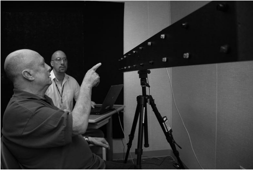
Figure 1. NVT scanner. A patient shown with a therapist in front of the light bar, with the therapist controlling the scanner and recording results on the NVT laptop.
